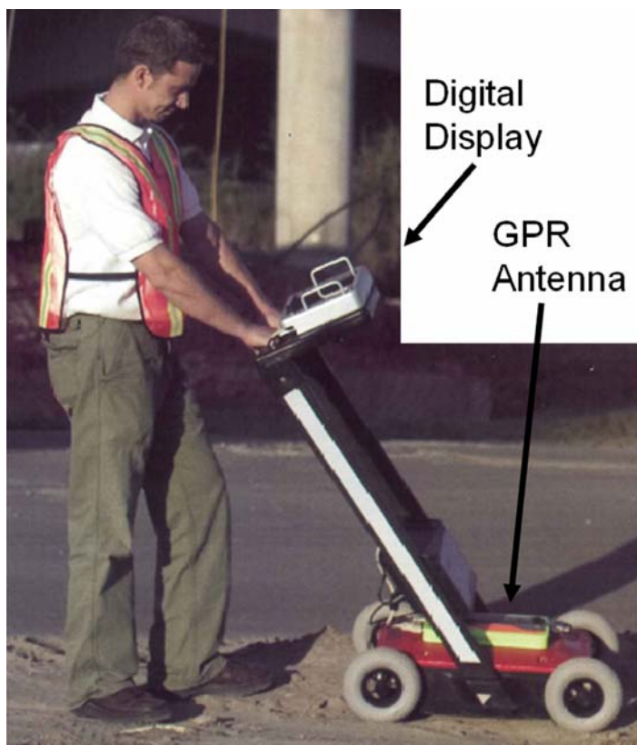
Figure 2.2: Photo showing GPR data acquisition using a commercially available digital display for data monitoring [13]. One user must simultaneously perform the two tasks of positioning the GPR antenna and monitoring the acquired data on the digital display. Results are displayed in profile view rather than a more intuitive map view.
